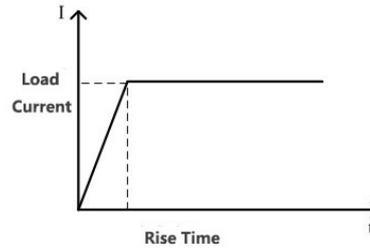
Figure 3- 8 constant current soft starting mode
