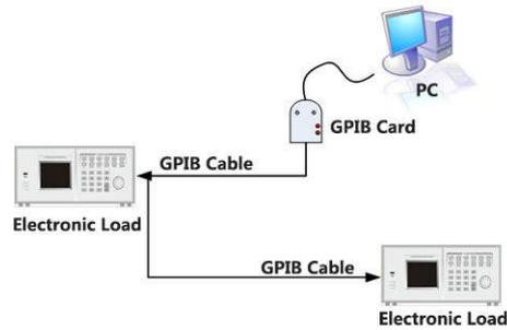
Figure 5- 1 GPIB system
