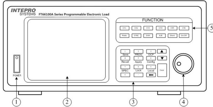
Figure 1- 1 Front Panel of Electronic Load
