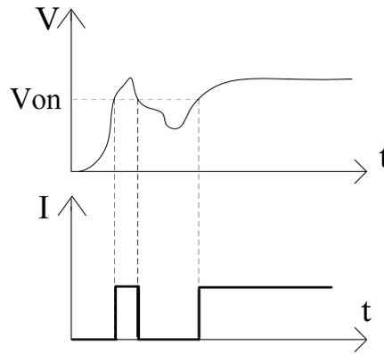
Figure 4- 4 Current waveform when Von Latch On
