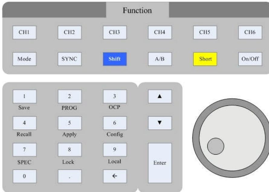
Figure 4- 1keypad of electronic load
