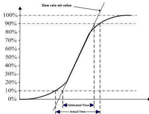
Figure 3- 15 relationship between slew rate and actual conversion time
