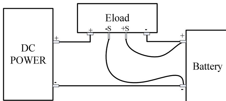
Figure 3- 12 battery charging test wiring diagram
