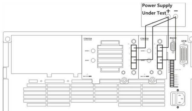
Figure 2- 5 load parallel line connection
