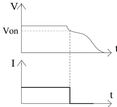
Figure 3- 14 Von Unloading (Von non-locking)
