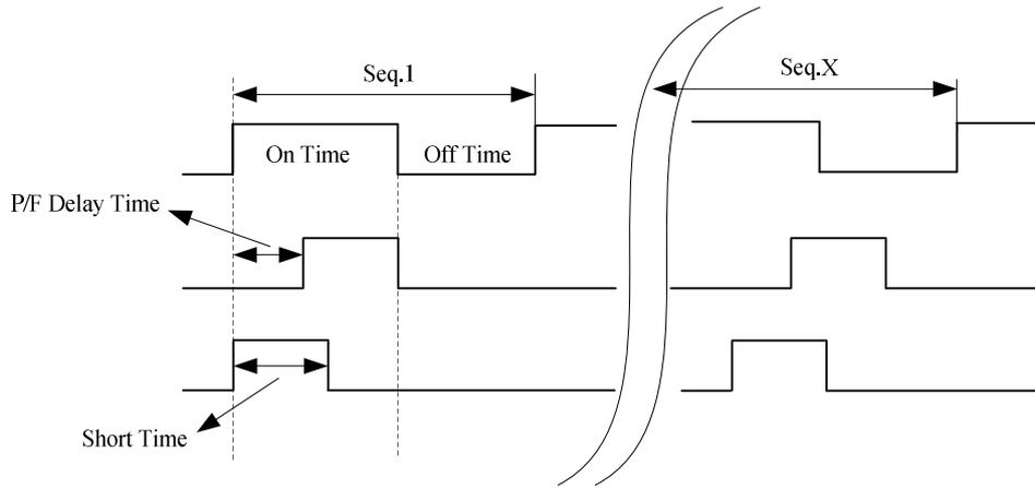
Figure 4- 2 Sequence when the program operates
