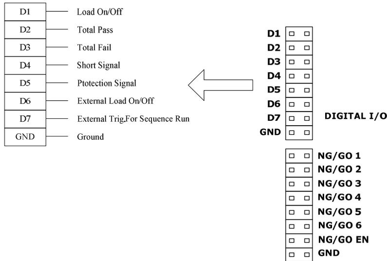
Figure 4- 5 Load control connection terminal
