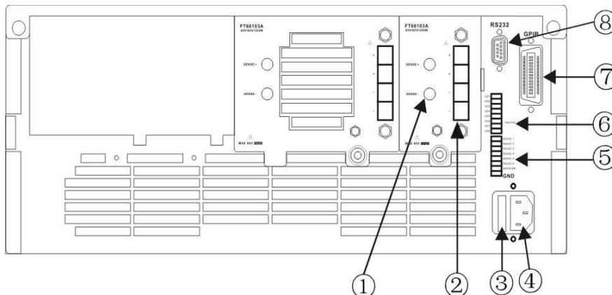
Figure 1- 2 Rear Panel of Electronic Load
