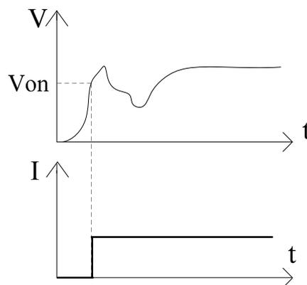
Figure 4- 3 Current waveform when Von Latch On
