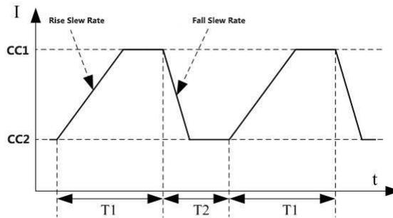
Figure 3- 3 transient constant current mode
