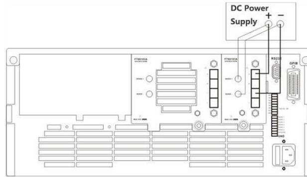
Figure 2- 4 remote sampling line connection
