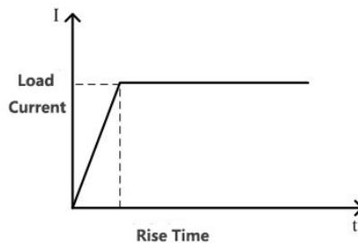
Figure 3- 9 constant current soft start mode
