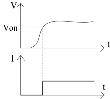
Figure 3- 13 Von Loading (Von non-locking)
