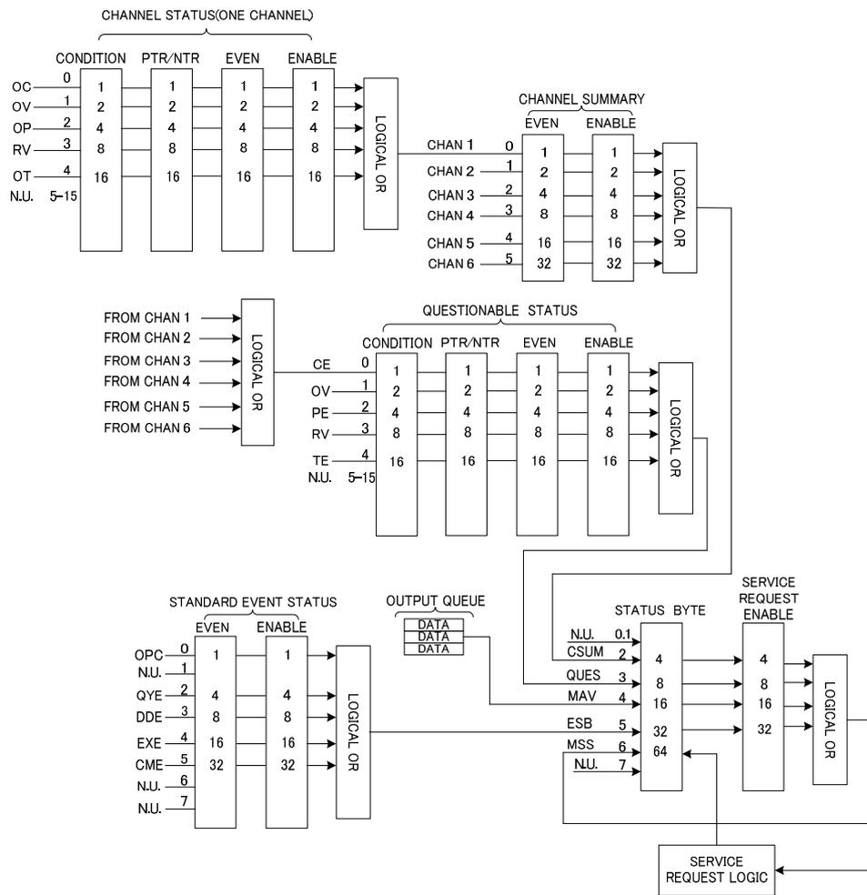
Figure 8- 1 Status register of electronic load
