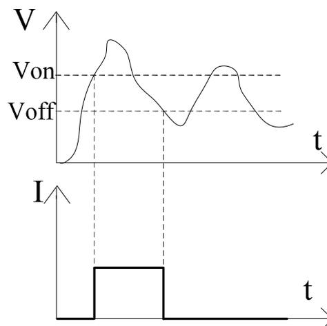
Figure 4- 4 Set load current waveform of Von and Voff
