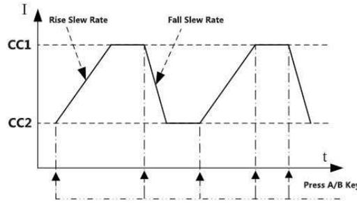
Figure 3- 2 steady state constant current mode
