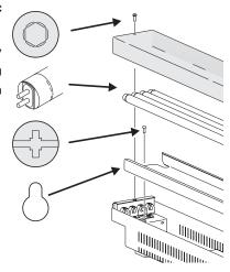
3 Using a Phillips screwdriver, loosen the two screws holding the cover of the wiring housing in place; remove the cover. To ensure adequate ventilation, we recommend that the Cyclo be installed with a minimum of 25 mm (1 inch) of free space on each side. Screw the fixture into place using, either:
