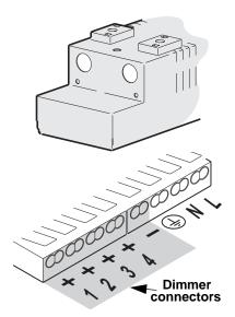
there are fewer connectors on Cyclo models with fewer than four tubes.) Connect the ground (earth) lead to the - terminal. Connect the other leads to the appropriate connectors. Notes that there are two connectors at each position and that you can use either one of these.
