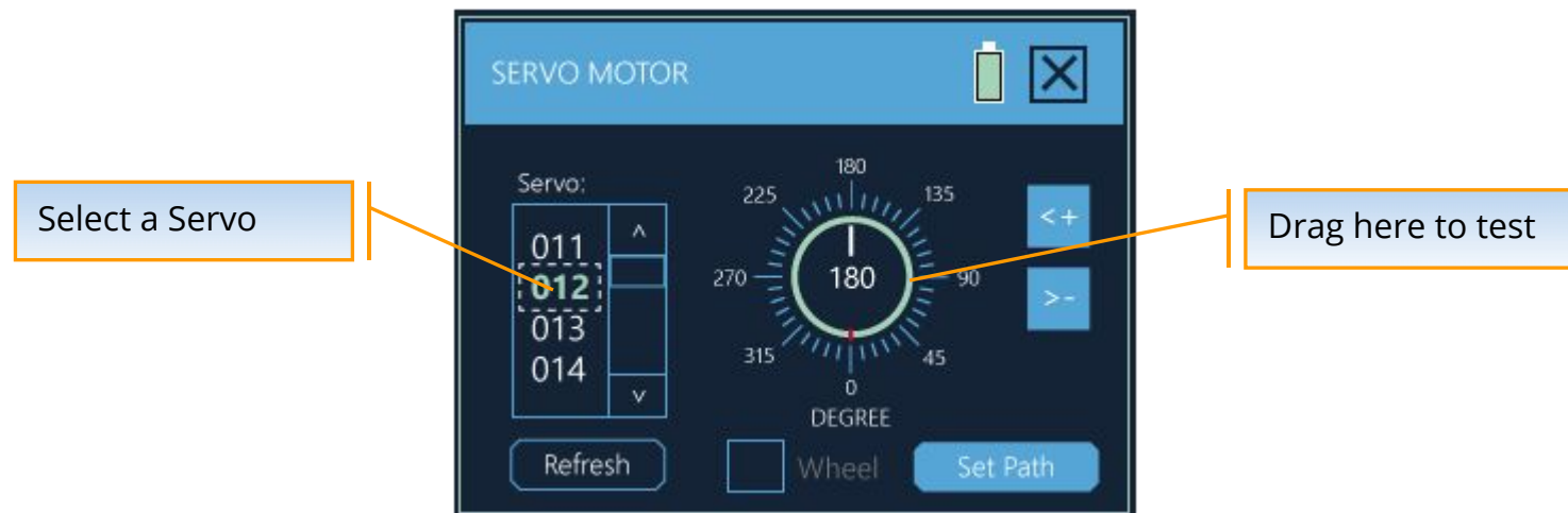
Testing Cube Servo with rero Controller
