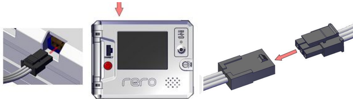
Connection to rero controller, connection between cube servo or sensors
