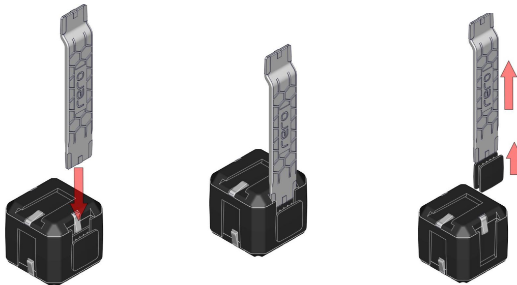
Release rero Interconnect from Cube Joint slot
