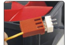
Connect the RPM Signal Connector to the Fan Connector
