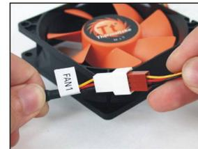
Above application shows Fan1 Fan Control Cable connected to a most common fan connector. This setup will allow Hardcano 13 to adjust fan speed and receive RPM signal as well.
