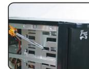
Secure the Hardcano 13 into any open external 5.25" drive bay with the screws provided in the package.
