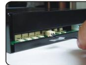
Connect the 2 pin connector of thermal sensor cable to the 2pin socket of Hardcano 13. You may place the **Thermal Sensor Probes** to different chassis locations.
