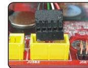
Connect the USB signal cable to the USB socket on Motherboard
