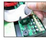
3.Plug the new battery into the socket
