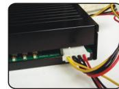
Connect the 4 pin MOLEX connector from computer power supply to the 4pin socket of Hardcano 13.
