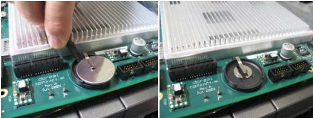
Figure 25: IMB Battery Removal
