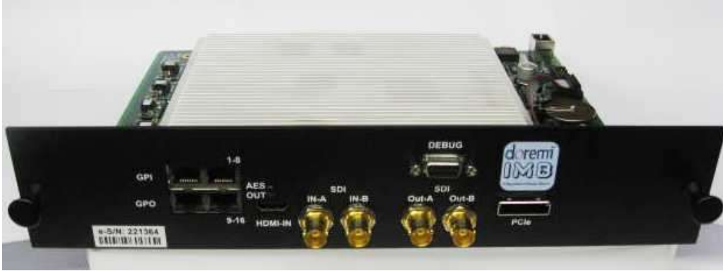
Figure 5: IMB Board With Barco Mounting Bracket
