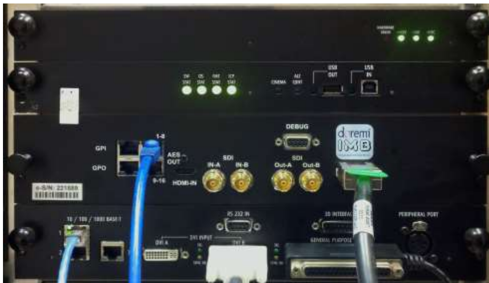
Figure 11: Barco Series-2 Projector with IMB Installed
