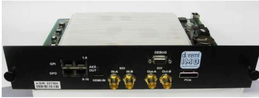
Figure 3: IMB with Barco Front Panel
