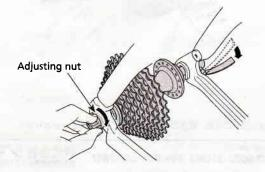
If the clamping strength is adjusted too strong and the quick release lever cannot be pushed to the CLOSE position, turn the adjusting nut in a counter-clockwise direction to reduce the clamping strength. When doing this, do not fully release the adjuster nut. Turn it 1/8 of a revolution, and then try to push the lever to CLOSE, to set the maximum clamping strength with which you can push the quick release lever to the CLOSE position.
