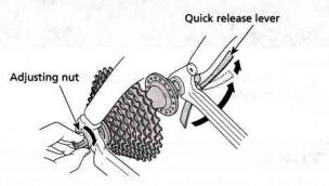
3. Grip the rear end with your fingers and use the palm of your hand to close the quick release lever with as much strength as possible. When closed, the quick release lever must be in the "CLOSE" position shown below in the diagram on the right. The side of the lever with the inscription "CLOSE" must be facing away from the bicycle, and the lever should be parallel to the rear end as shown below in the diagram on the left.
