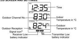
\* When the signal from the transmitter is successfully received by the Temperature Station, this icon will be switched on. (If not successful, the icon will not be shown on the LCD). User can therefore easily see whether the last reception was successful ("ON" icon) or not ("OFF" icon). On the other hand, the short blinking of the icon shows that a reception is being done at that time.
