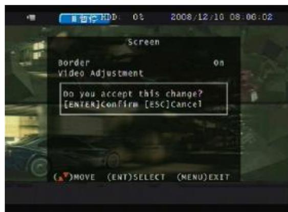
After adjusted, press ENTER to see if it has change the dialogue resolution, press ENTER to change, press ESC to cancel. If user does not make any change, the mode will change back to last status after 15 seconds.
