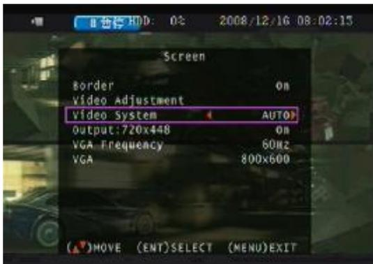
Auto as the default, users connect any video input to channel 1 and then power on DVR to detect video system.
