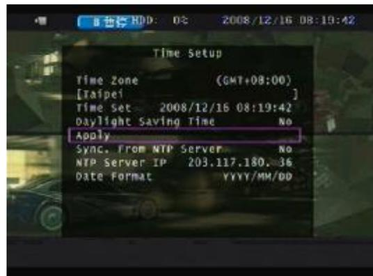
Select time zone and auto time synchronization with NTP server. Network is required on NTP server. After time set or daylight mode turns to on, user needs to Apply and confirm. 0 ~ 9 is repeatable with increase + button,
