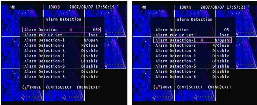
Alarm Signal type depends on Alarm Sensor polarity define on NO (N/Open) or NC (N/Close) mode. Alarm POP UP: Event channel jump to full screen when alarm triggered. 9 Split screen with the alarm symbol if there is more than two cameras triggered.
