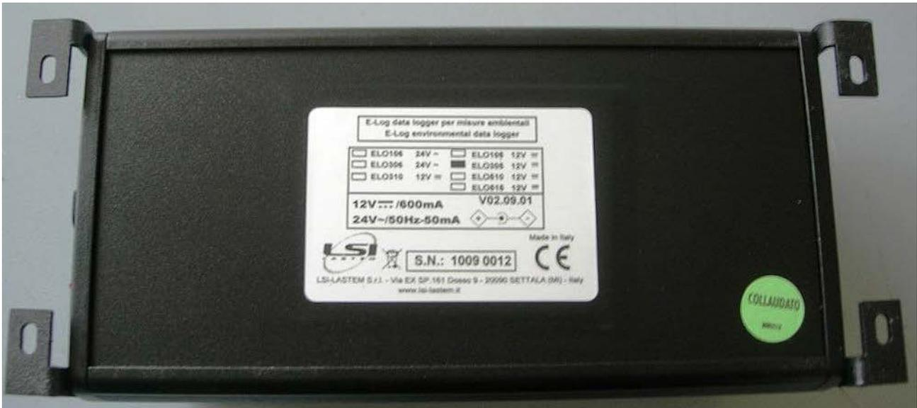
Figure 16: Nameplate of the Meteo Center weather station
