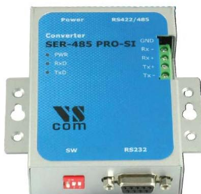
Figure 12: RS232-RS485 converter
