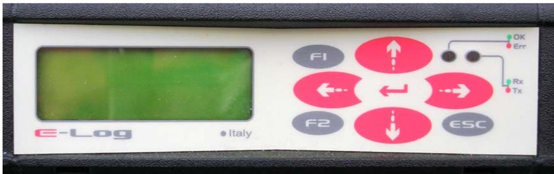
Figure 14: Front part of the datalogger
