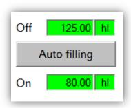
Two point controllers are used where a range and not a fix limit is used.
