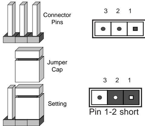
**Note:** On two pin jumpers, "Closed" means the jumper is on and "Open" means the jumper is off the pins.
