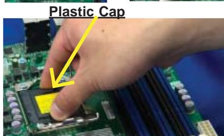
Hold the north & south edges of the plastic cap to remove it
