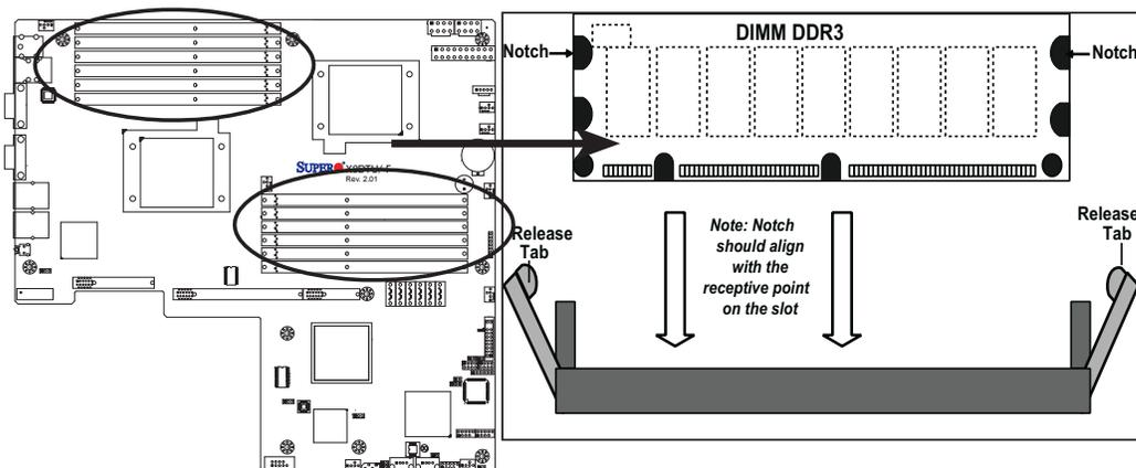
**To Install:** Insert module vertically and press down until it snaps into place. Pay attention to the alignment notch at the bottom.
