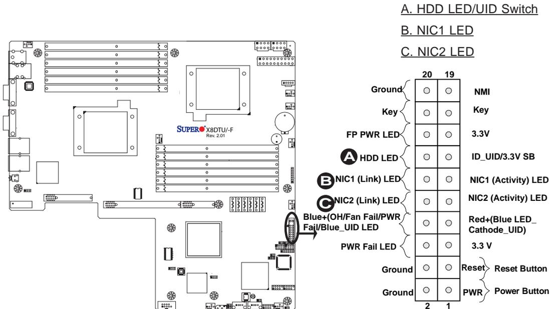
**Overheat (OH)/Fan Fail/PWR Fail/UID LED**
