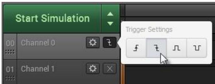
After setting the trigger, you can press the start button to begin searching for the trigger. If and when the trigger condition is identified, data collection will start.
