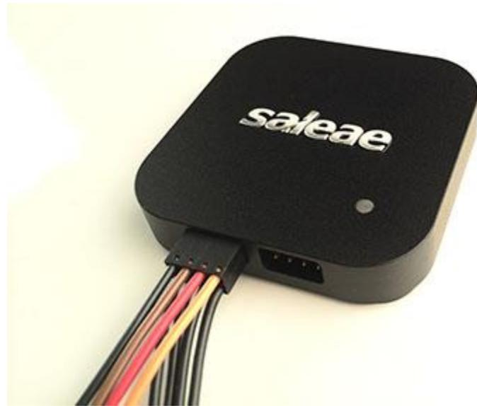
Note that the test lead color matches the channels in the software. The colors reflect the resistor color code for numbers 0-7. The numerical channel number is written on the white heat shrink at the ends of the leads. The lead ends are terminated with a Molex 0016020086 crimp connector for connection to typical .100-inch spaced headers/pins. The 2x4 plastic housing is Molex 0022552081.
