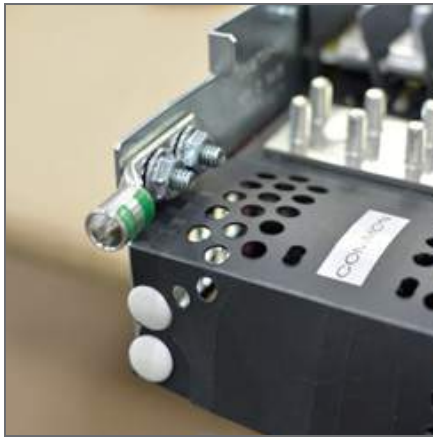
Left Ground Connection
