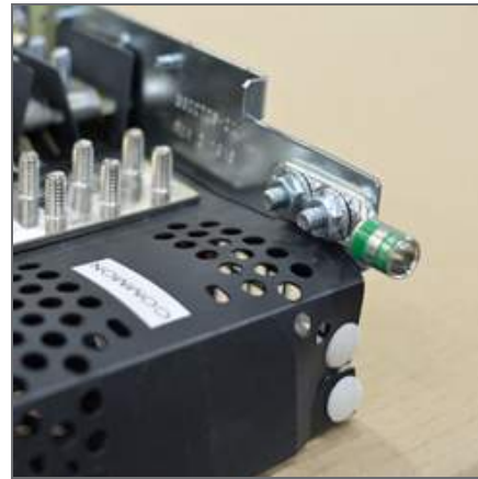
Right Ground Connection
