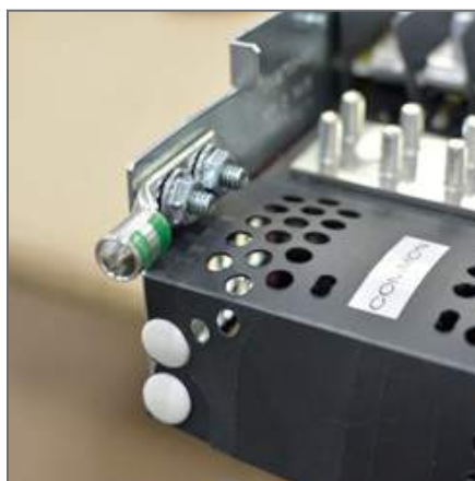
Left Ground Connection
