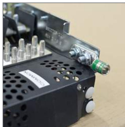
Right Ground Connection
