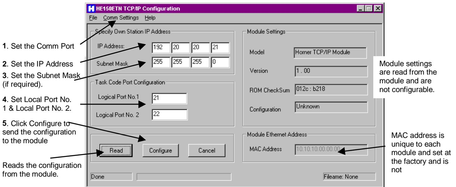
Figure 2.1 – HETCPIP Configuration Software Screen
