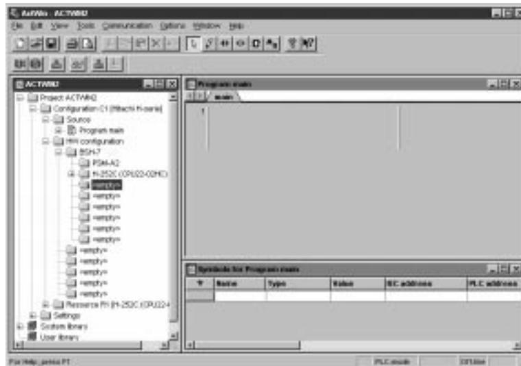
Step2: Right click on the appropriate <empty> slot under HW Configuration in the project tree. Select the "add module" command from the pop-up menu to create a hardware configuration with a CPU and an input module and output module.
