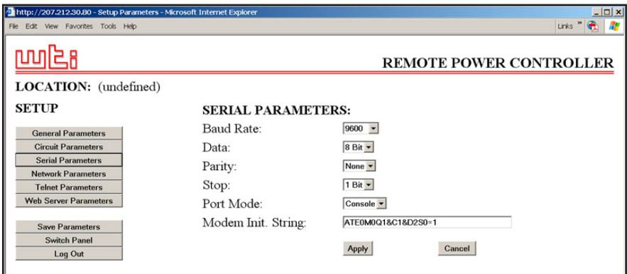
Figure 5.5: Serial Parameters Menu - Web Browser Interface
