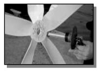
The air hub features concentrically arranged conical pins. Identify the matching conical recess in the turbine blade assembly and offer the turbine hub up to that side, aligning the pins with the recesses. Finally, to complete the assembly, screw the clamping plate onto the hub and tighten firmly.
