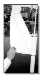
In wind mode, as with all wind turbines, the major hazard lies in accidental contact with the turbine blades. Although DuoGen's blades run more slowly than many competitor machines, they are still capable of inflicting injury.
