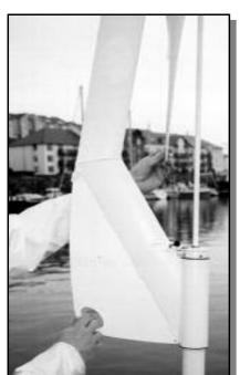
To stop DuoGen wind mode, grasp the yaw arm handle and turn the machine gently through 180°. The turbine will slow down and stop. As soon as it stops, grip a turbine blade to prevent rotation (the blades will run backwards down wind!). Release the spring plunger and lower the yaw
