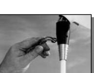
Withdraw the drop nose pin and disconnect the drive shaft.
