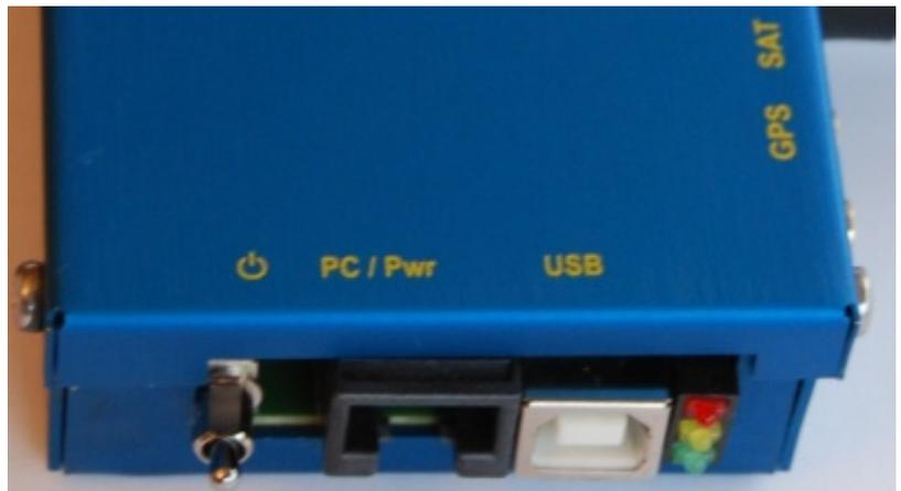
The RJ45 is the one to be used to connect the system to a PC for using the DSX software or any other software approved by DSX (please see the [www.d-s-x.net](http://www.d-s-x.net) page for the list). This socket can also be used to take the data output from the SAFLY (GPS navigation and other proprietary sentences) and to send to the SAFLY data for configuration and transmission.
