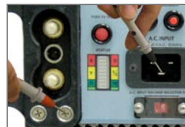
3.8.8 - Positive Probe to the Fastener Screw on the DC Receptacle.
