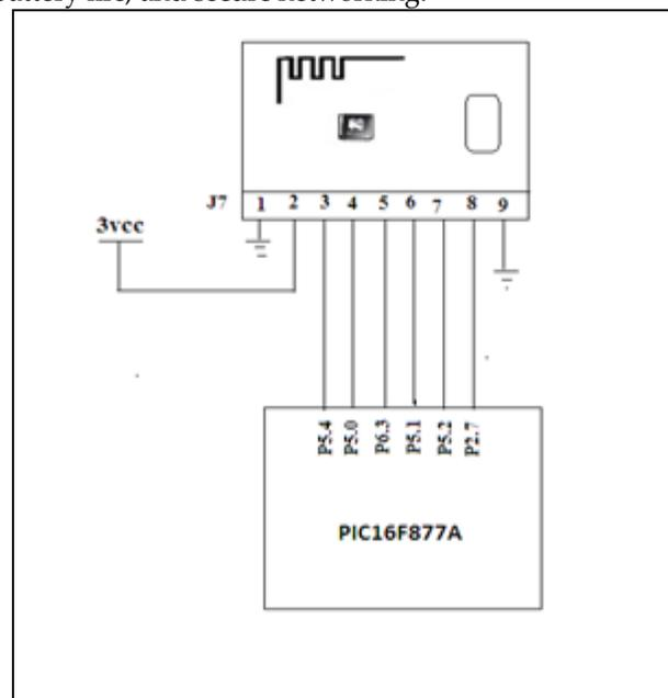
**Fig 1 ZIGBEE SENSOR AND PIN CONNECTIONS**
