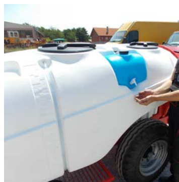
This symbol identifies the clean water tank on the machine used to wash your hands
