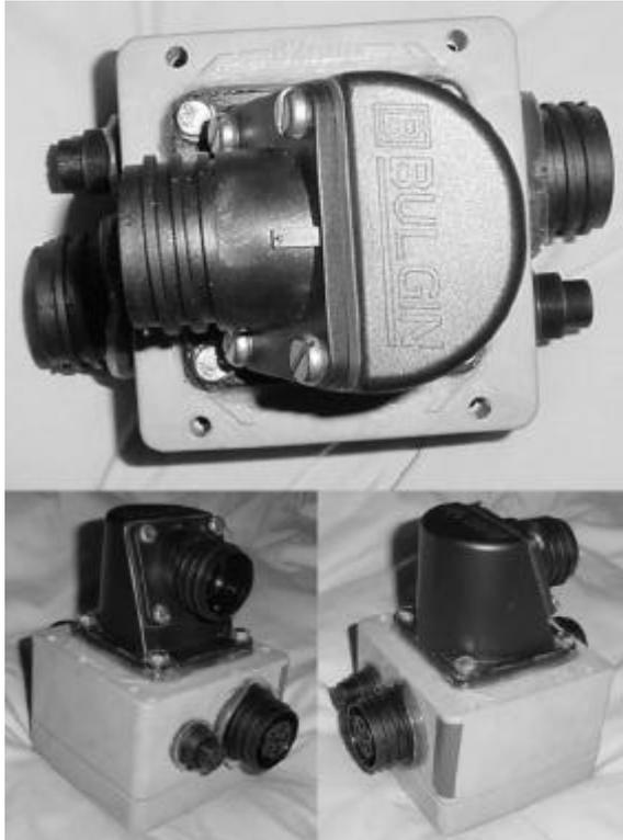
**Figure 82 - The location of the connectors on the main circuit enclosure**
