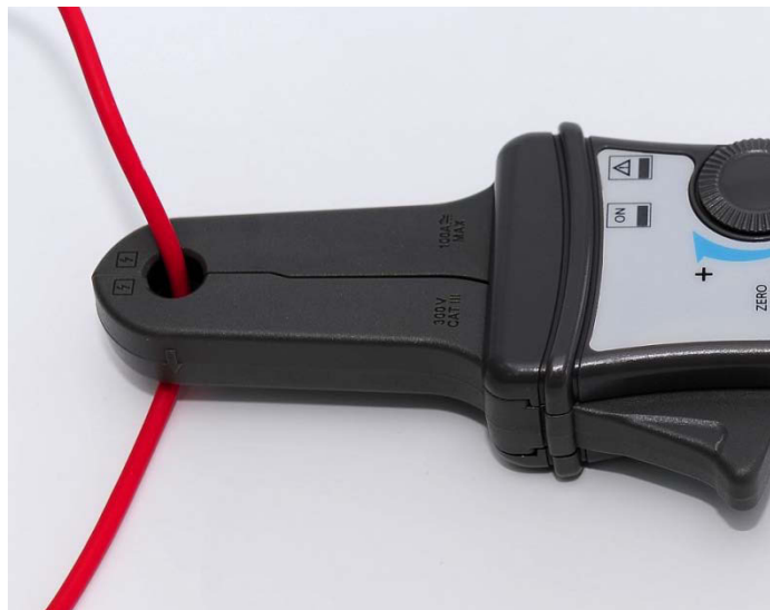
Figure 5: Connecting the CP62 current probe.
