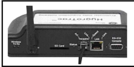
**Note:** *The modem interface is surge protected by a non-replaceable non-resetting slow-blow fuse. If you use a phone line that experiences frequent surges or lightning strikes, you should put a surge protector in line with the phone line to protect the modem from damage.*
