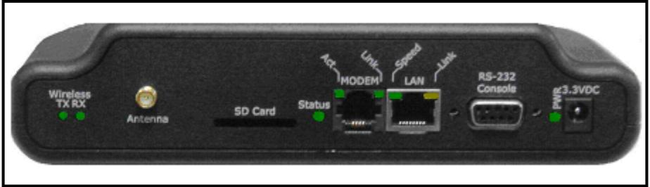
Figure 3: Data Acquisition Gateway - Rear Panel LED Detail
