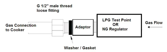
Adaptor must be fitted on gas connection to cooker prior to assembling other components. For NG, connect the natural gas regulator with the integral test point by using approved gas thread tape.
