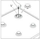
Disassemble the worktop by unscrewing the rear screws. In this way it is possible to lift the worktop and to reach the inside components.
