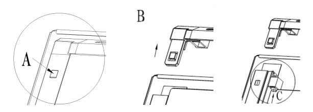
To remove the oven glass for cleaning, first press clip A on left and right side down simultaneously, and pull according to direction B. The cover is now removed and inner glass could be taken out now.
