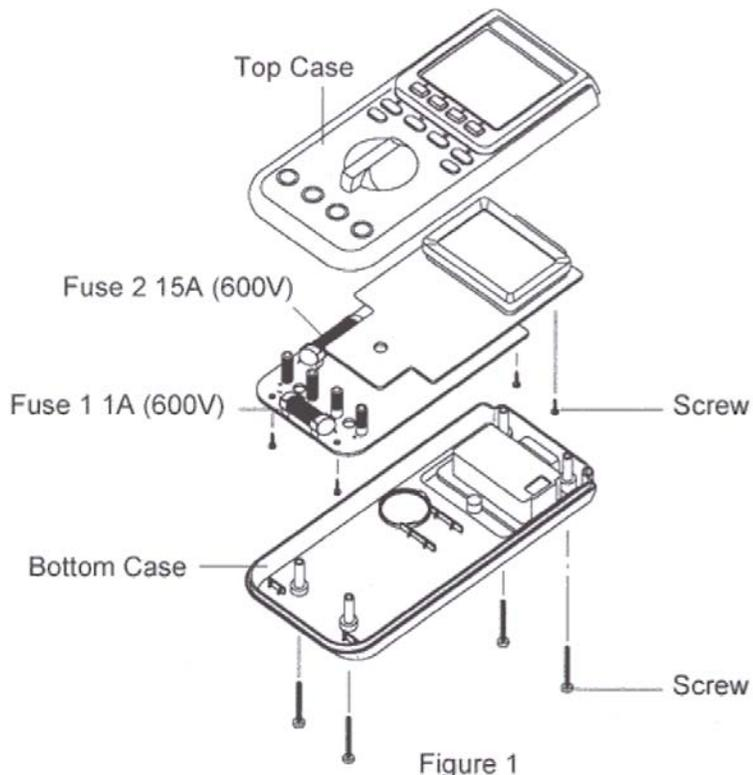
**WARNING: Installing improper fuses can cause injury and product damage**
