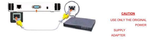
**STEP 3.** Connect the power adapter.
