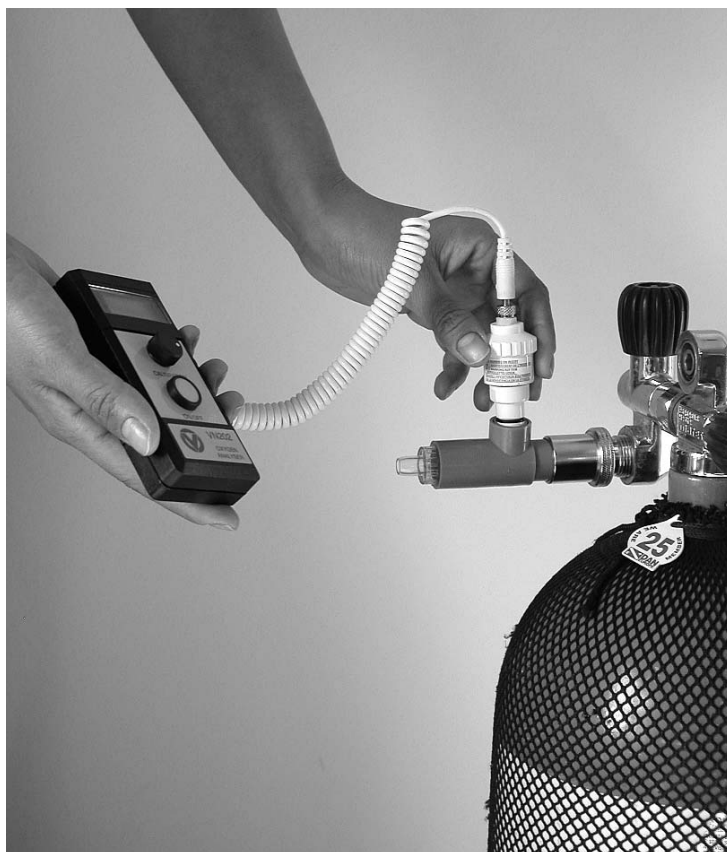
Device to check the flow of Nitrox on the sensor of the analyser
