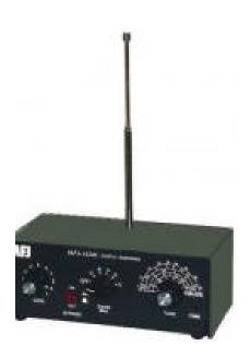
MFJ invented the tunable active antenna! New technology uses dual gate MOSFET and a gigahertz bandwidth buffer
