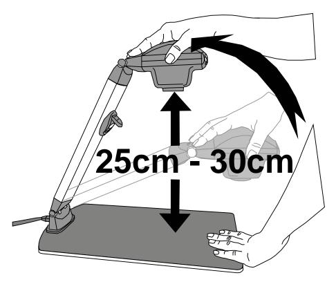
Raise the camera so that it is roughly 25 to 30 cms above the table. If it is too far or too close to the text the camera will not be able to focus correctly.
