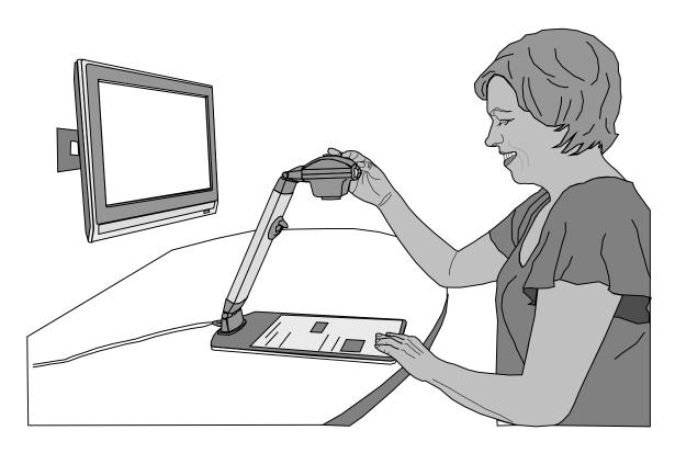
Place the material you wish to read on the reading table, looking at the TV screen to see where you are. Adjust the magnification to suit. Ensure the camera head is horizontal for optimum image quality.
