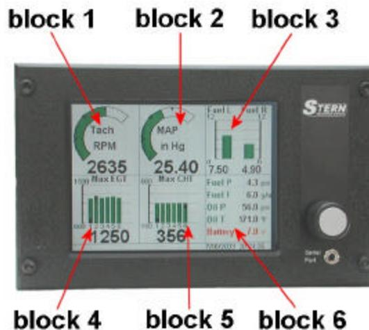
Figure 1.3: Each normal operation display page has six blocks
