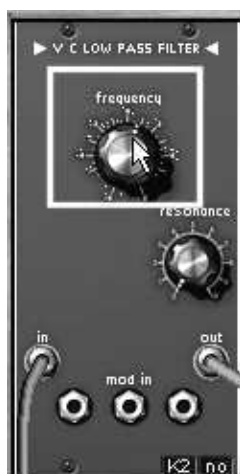
The setting of filter1 cut-off frequency
