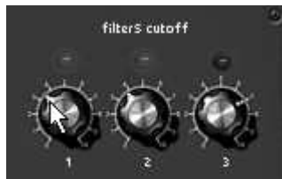
The three filter cutoff frequency controllers
