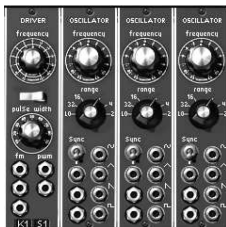
An oscillator bank (1 "driver" and 3 "slave oscillators")
