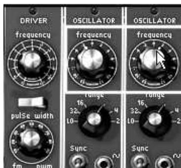
Detune the pitch of the second oscillator
