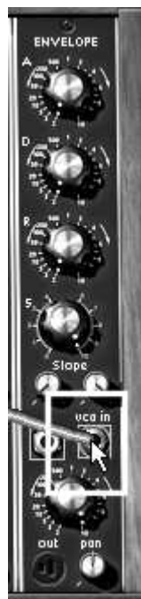
Connection of the VCA2 audio input
