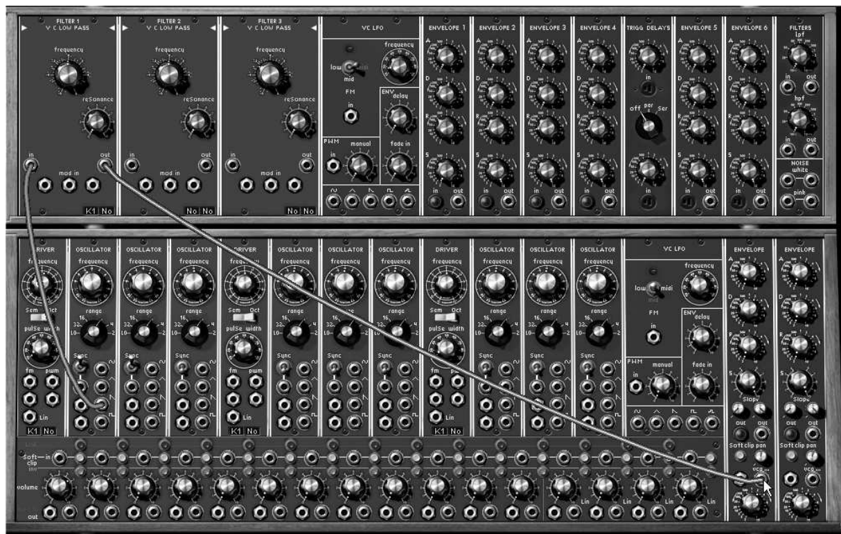
Connection of the filter1 audio output to the VCA1 audio input
