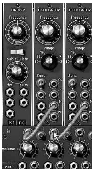
Connection of oscillators to mixer
