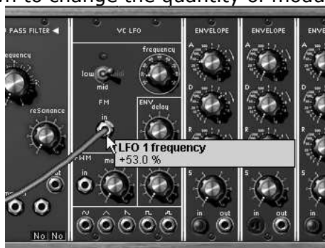
Setting the modulation quantity
