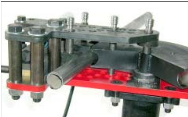
Figure 26 - Die set installed as seen from back side of bender
