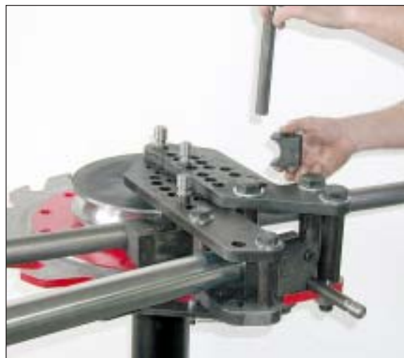
Figure 25 - Installing pin in back hole
