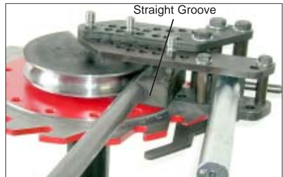
Figure 21 - Pressure Die installed - front
