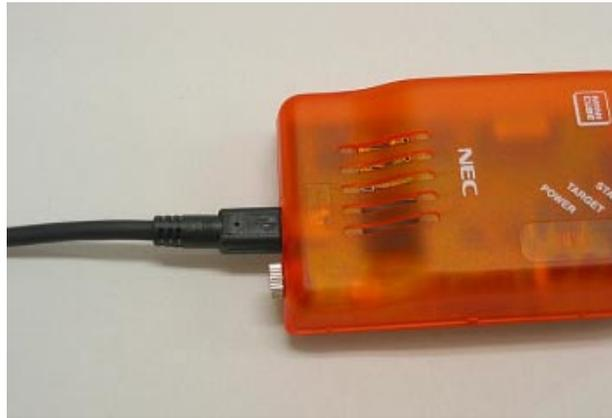
**(4) USB interface cable connection (host machine side)**
