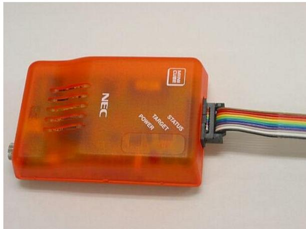
**(2) Attach the QB-78K0MINI connection cable (self-check board or target system side)**
