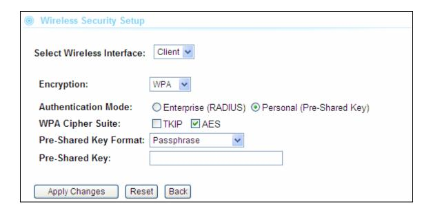
■ Encryption Type: There are two encryption types TKIP and CCMP (AES). While CCMP provides better security than TKIP, some wireless client stations may not be equipped with the hardware to support it. You can select TKIP and AES to allow TKIP clients and CCMP clients to connect to the Access Point at the same time.
