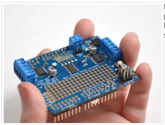
Finally, break off a 2-pin piece of header and place it next to the POWER terminal block, short legs down, tape it in place if necessary and solder it in.
