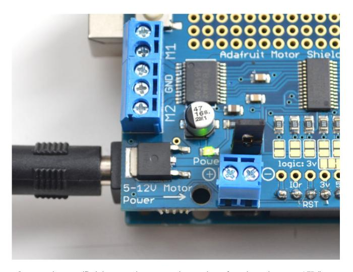
Once you have verified the motor is connected properly **and** you have the power LED lit up brightly, we can upload our code.
