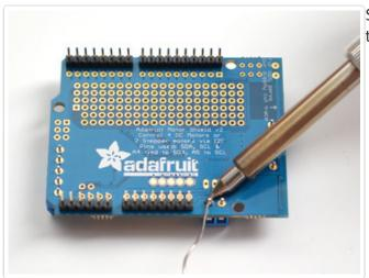
Solder in the two pins of the external power terminal-block
