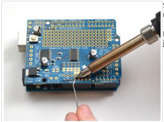
Solder each one of the pins into the shield to make a secure connection
