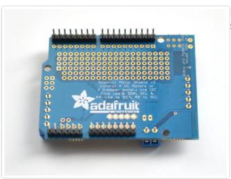
Flip the board over so that you can see & solder the pins of the terminal blocks
