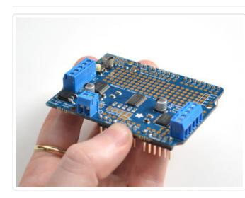
Next we will install the terminal blocks. These are how we will connect power and motors to the shield. They're much easier to use than soldering direct, just use a small screwdriver to release/attach wires!
