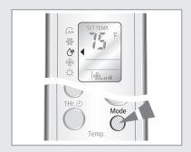
2 Press the ∩ button on the remote control until 🗗 is displayed.
