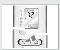
3 Press the  $\nabla \mid \triangle$  button to adjust the temperature until the required temperature is displayed.
