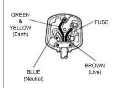
The wire which is colored **BLUE** must be connected to the terminal which is marked with the letter N or colored Black. The wire which is colored **BROWN** must be connected to the terminal which is marked with the letter L or colored Red.
