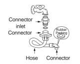
(3) Connect the inlet hose adapter to the water inlet of a washer and turn it to be fixed.
