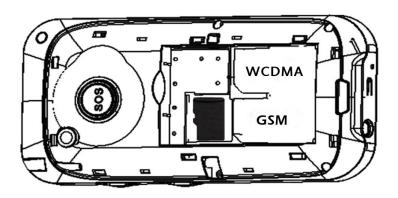
Install battery and replace battery cover.
