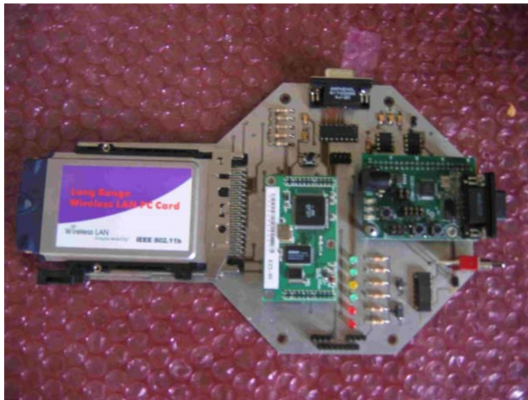
Figure 3. First generation wireless printed circuit board, which attaches to the robot as a daughter board.
