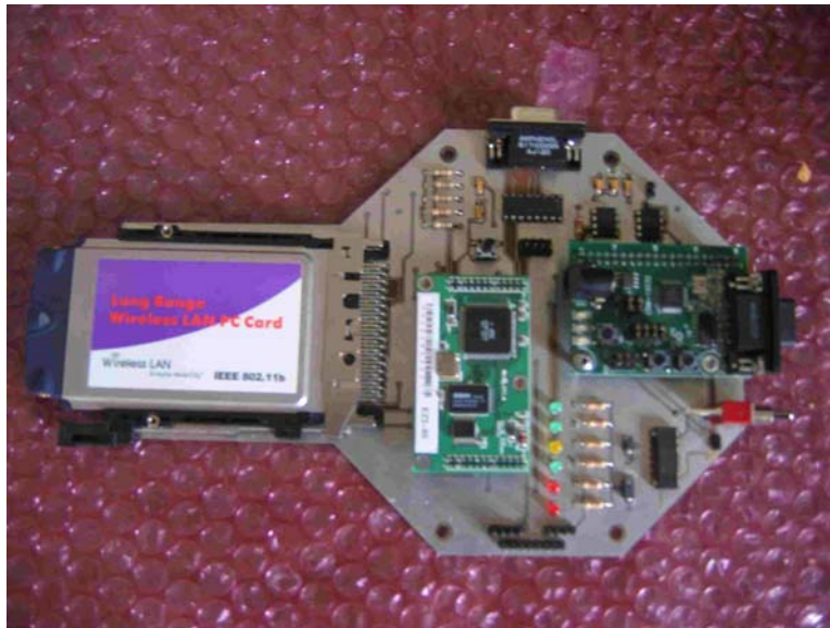
Figure 9. First generation wireless daughter board with PCMCIA card, EZL-80 and CSM modules installed.
