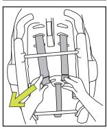
3 Remove the seat cover from the adjustment button as shown.
