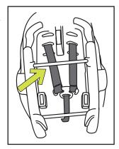
They must not must pass over the outside of the steel bars at the back of the restraint.
