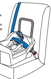
Use the Belt Path labels as a guide for correct belt placement.
