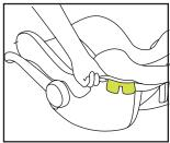
2 Remove the harness from the splitter plate.
