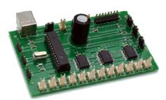
The card can be configured with dedicated software via USB and store in internal eprom memory the applicable maximum power for each channel and the power used by default when connecting. Variables can also be programmed using SIOC IOCP code.
