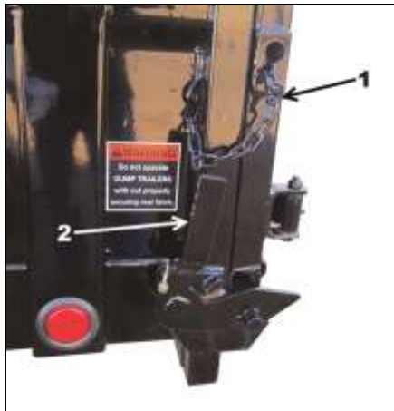
Set Metering Chains and Unlock Spreader Gate
