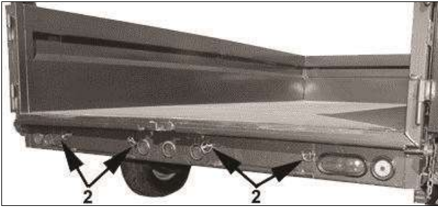
Ramp Safety Lock Pins
