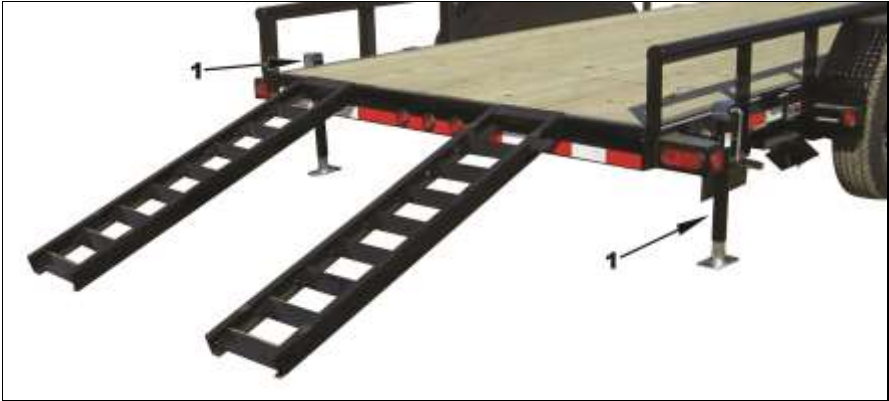
Rear Jack and Ramps
