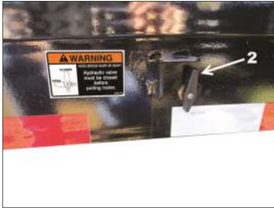
Deck Control Valve
