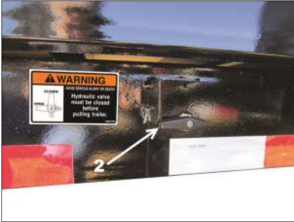
Deck Control Valve
