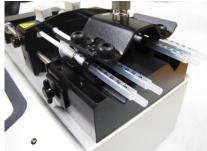
Figure 5. Four 1cc syringes secured in syringe rack (top) and secured onto pump (bottom).
