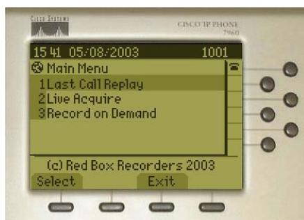
**DTMF Tones** - for Integrations supporting DTMF detection such as TDM Trunk side implementations, DTMF tones can be used to allow Record on Demand to function by pressing a specific key sequence on the phone during the call.
