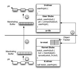
Figure 3. Data movement from the k-driver to the u-driver: (1) a call to the client stub of a u-driver function marshals the data structure; (2) kr-mod invokes the user thread and copies the marshaled data into user space; (3) ur-lib consults the object tracker and unmarshals the data structure; (4) ur-lib invokes the u-driver function on the unmarshaled data structure.
