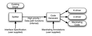
Figure 5. Architecture of DriverSlicer. The splitter infers a partition of the device driver, while the code generator produces the k-driver, the u-driver, and RPC code for data structures that cross the user/kernel boundary.
