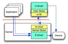
Figure 1. The Microdrivers architecture. The path for performance-critical functions is a solid line, and for non-critical functions is dashed.
