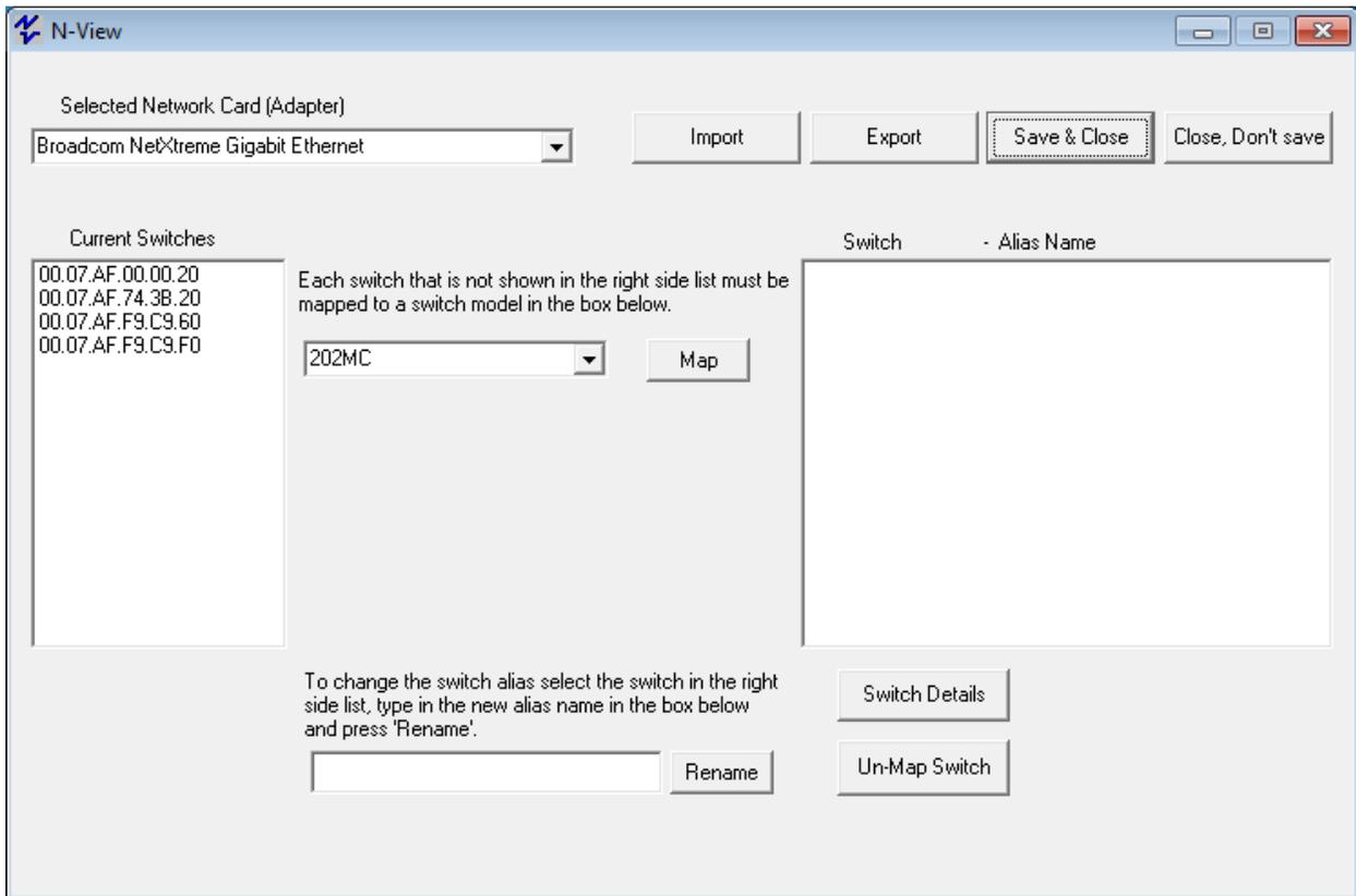
If the Network Adapter that is displayed by default is not the adapter to which the switches of interest are connected, then select the correct adapter.
