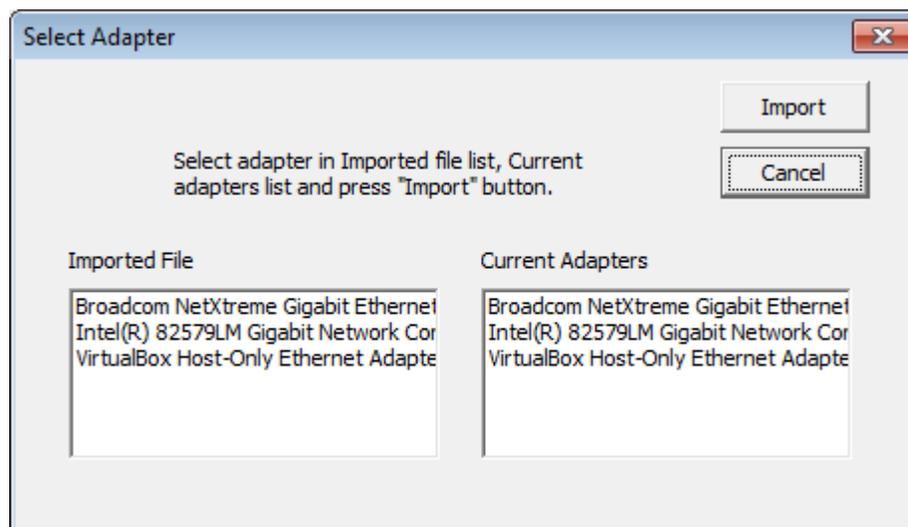
Select one NIC in each window to assign which LAN the mapped and aliased switches are coming from (on source PC) and going to (on target PC).
