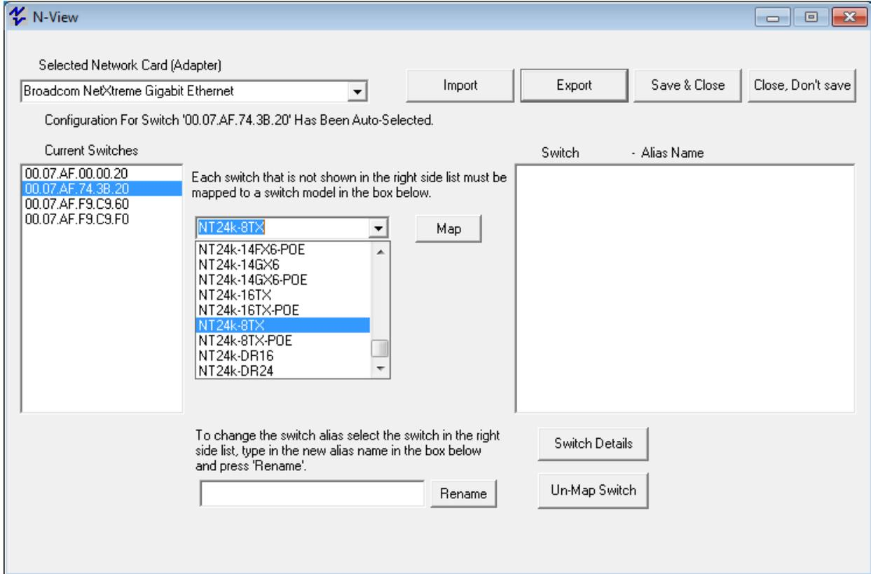
Several N-Tron switches report their model and configuration to N-View, and in those cases the switch model and configuration may automatically fill in the configuration values. These include all 700, 7000, NT24k and the –N and –A versions of several of the 500 series switches. Verify that these values are correct on both N-View and the switch before proceeding to map it. Note that the N-View values will reflect the user’s configuration for several switch versions.
