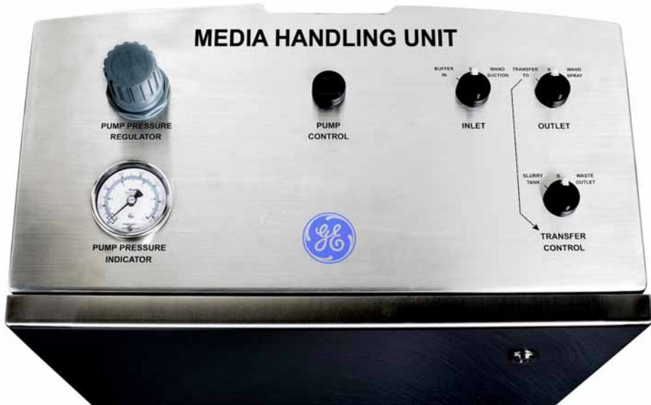
Fig 1-10. The layout of the control panel on the Media Handling Unit.
