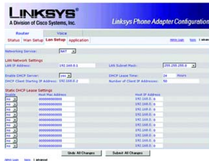
Figure 6-6: Router - LAN Setup Screen
