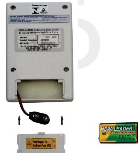
Figure 7. The 9 Volt battery connection. Type of battery used with device: IEC 6F22 - 9 Volts battery.
