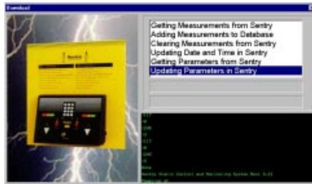
If for some reason the previous data downloaded from any of the Sentry units has been lost, this data can be retrieved **provided that no new measurements have been made**. In order to restore the data, perform a download as usual **but hold down the SHIFT key when you click on the Download button**.
